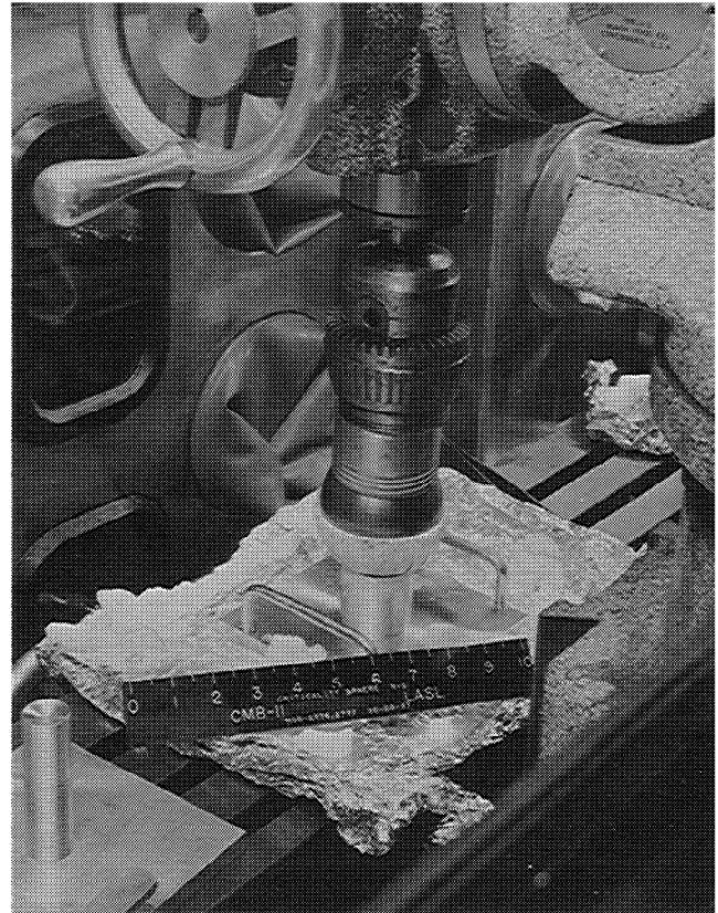
Fig. 2. Cooled lower hemisphere being shrink-fitted into self-heating upper piece.
