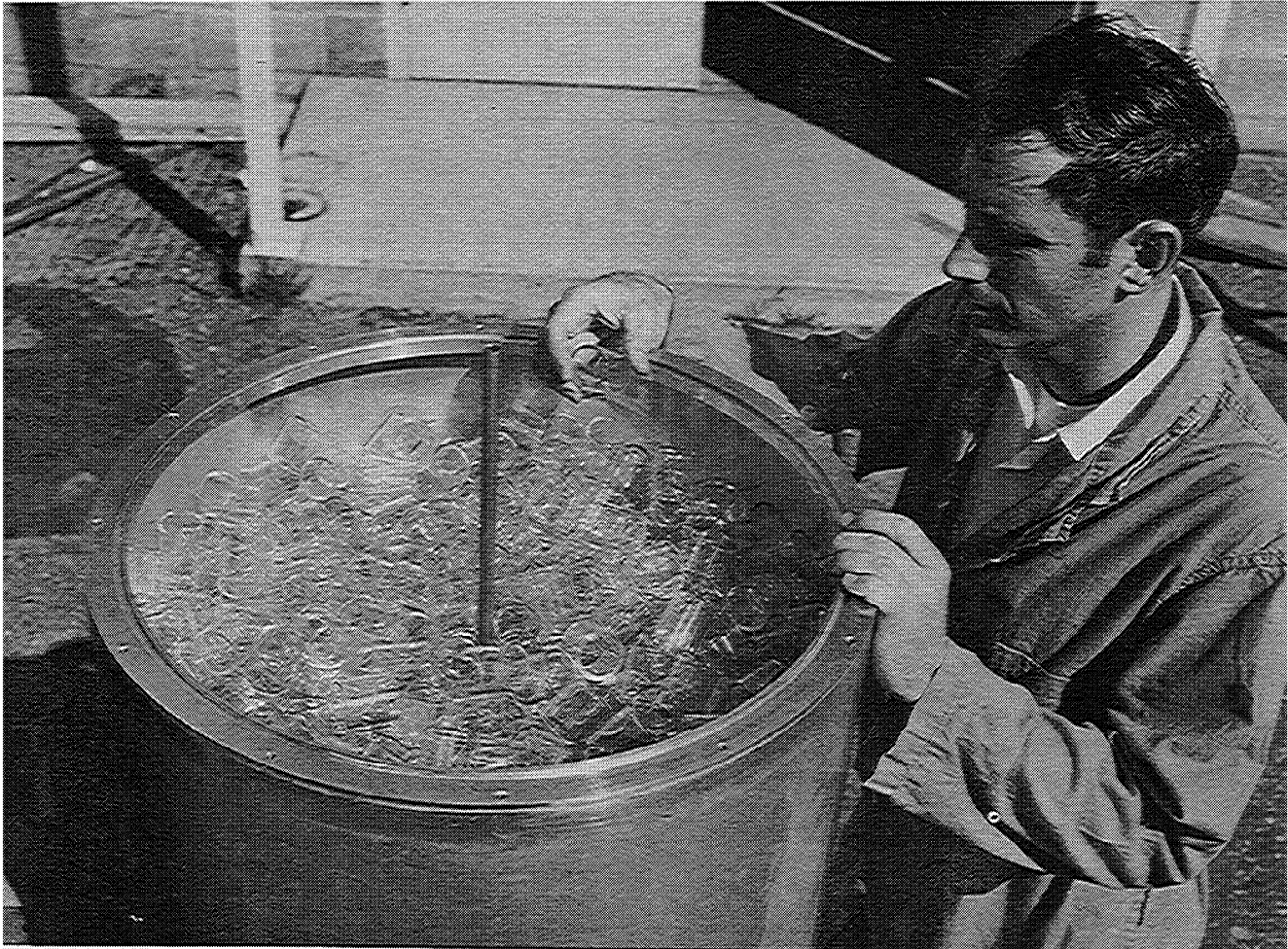
Fig. 2. Experimental vessel loaded with glass raschig rings.
